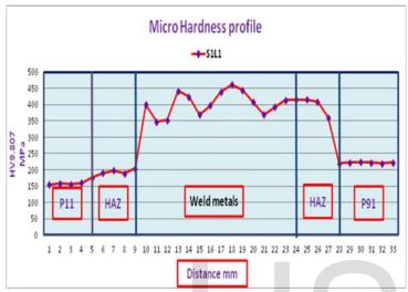
Figure 18. Hardness profile of dissimilar weld joint between P91 and P11steel with E9015B9/E90SB9 filler metals.
