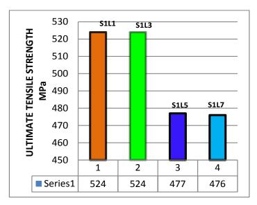
Fig.22. Ultimate tensile strength of different heat treatment Sample S1L1, S1L3, S1L5 and S1L7
