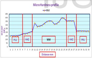
Figure 19. Hardness profile of dissimilar weld joint between P91 and P11steel with E9018B3/ER90SB3 filler metals.
