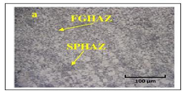
Fig.14a SPHAZ and FGHAZ 0.5 hour
