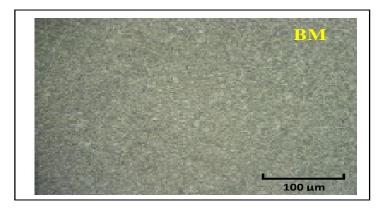
Figure 8 P91 base metal Microstructures after welding and intermediate PWHT
