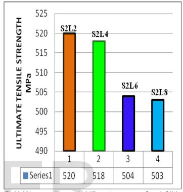
Fig.23. Ultimate tensile strength of different heat treatment Sample S2L2, S2L4, S2L6 and S2L8
