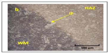
Fig. 4b Interface of P91 with weld metal
