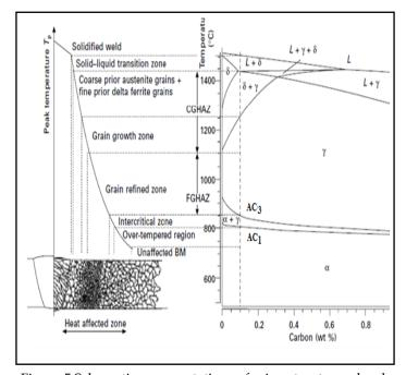
Figure 5 Schematic representations of microstructures developed in weld metal and HAZ as function of peak temperature
