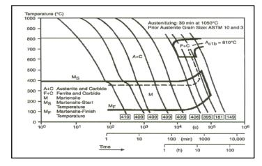
Figure 6 CCT diagram of steel P91[6].
