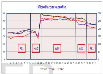
Figure 20. Hardness profile of dissimilar weld joint between P91 and P11steel with E9015B9/E90SB9 filler metals at 750°C 0.5hr, 1hr and 2hrs.
