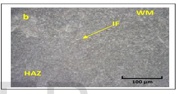
Fig. 9b Interface of P91 with weld metal
