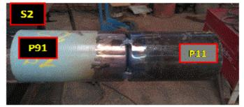
Fig. 1 Weld joint between P91 and P11 Pipe (a) Sample 1 (b) Sample 2
