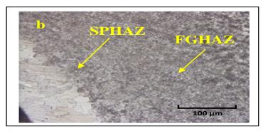
Fig.14b SPHAZ and FGHAZ 1 hour
