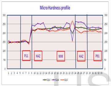
Figure 21. Hardness profile of dissimilar weld joint between P91 and P11steel with E9018B3/E90SB3 filler metals at 750oC 0.5hr, 1hr and 2hrs.
